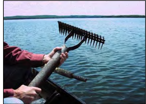
Endangered Resource Services used a rake (pictured above) to collect plants for the plant surveys. Rake fullness is a measure of plant density.
